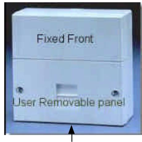
When the front screws are removed the complete lower portion of the socket including the IDC connectors for user wiring can be pulled out. They connect to the back plate by means of a fixed plug. The fixed plug is a standard BT plug and socket and allows all the internal wiring to be easily isolated for fault finding. A normal phone can be plugged directly into the socket remaining in the wall to test if the line is OK.
