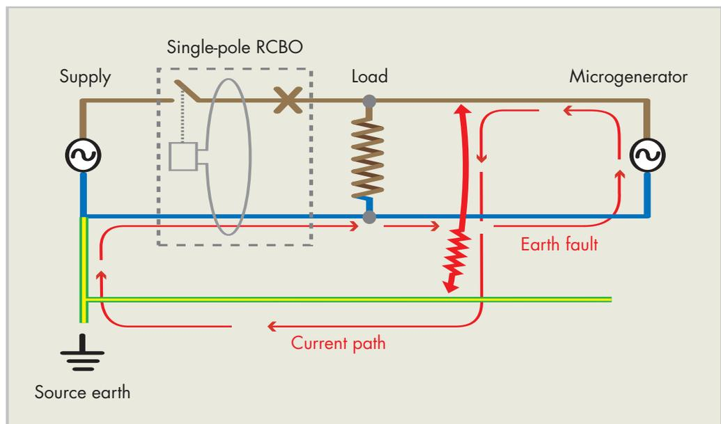
It should be noted that, if the RCD element of the RCBO has been provided for additional protection against electric shock, this arrangement is not permitted and the RCBO would need to switch both line and neutral conductors (see (ii) above).
