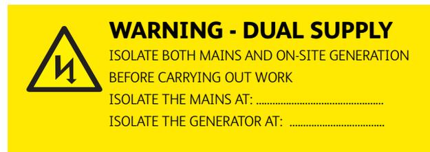
In addition, G83/1 and BS EN 50438 require up-to-date information to be displayed at the point of connection with a distributor's network as follows:
